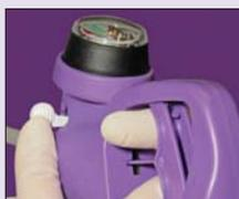
Figure 4 - Vacuum release lever
